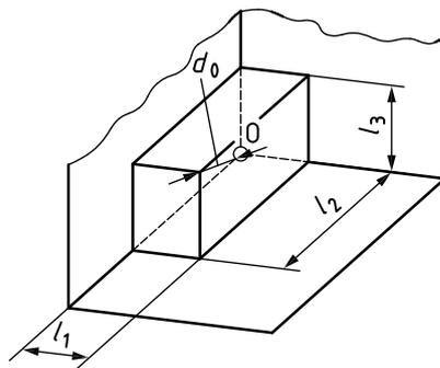
c) Reference box on three reflecting planes,  $d_0 = \sqrt{l_1^2 + l_2^2 + l_3^2}$
